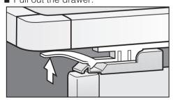
■ Raise the snap fittings on both sides and lift the drawer out.
